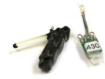
Satellite Telemetry- A transmitter is attached to the bird. The transmitter sends its signal to an orbiting satellite. The satellite re-transmits the data to a receiving station, which researchers then access through their computer.
